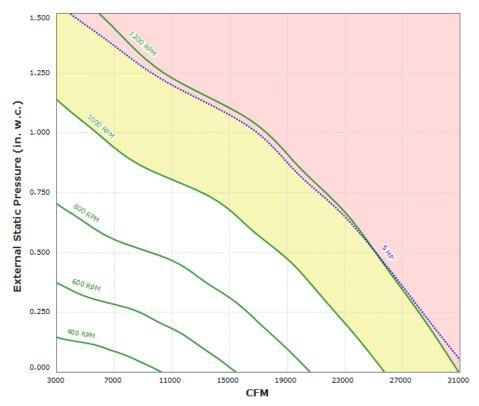
Max Sizeable RPM = 1200 RPM. Curve shown extended beyond this point for reference only.
